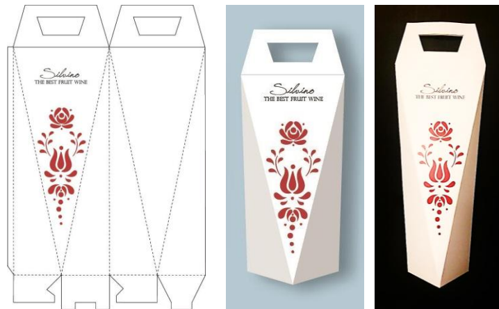
Figure 5: Technical drawing of the selected packaging design decorated with Hungarian folk art motif, the virtual and the paperback prototype by Wolford Diana, 2017. Tutor: Dr. Edit Csanák (DLA)
